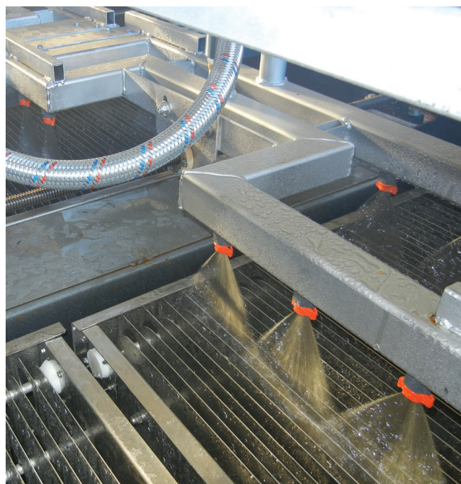
Automatic cleaning system of the filter: in detail, the washing manifold, mobile by means of gearmotors and the nozzles that allow the complete washing of electrostatic cells and mechanical panels. Pollutants are collected in the tank integrated in the filter.
