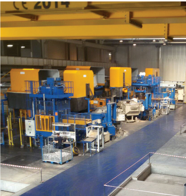
■ Hoods into two parts on COLOSIO PFO die-casting machines of different tonnages connected to a centralized suction and filtration system ENERPROG - Russia
