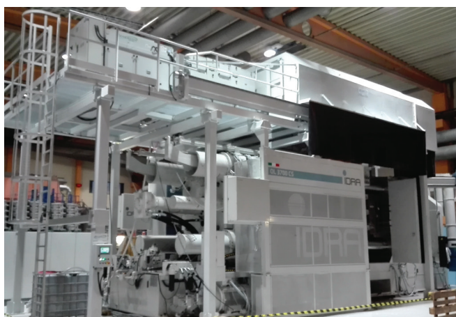
■ Hood into two parts complete with individual ENERPRESS suction and filtration system for recirculation of purified air in an environment on IDRA OL3700CS die-casting machines - Sweden
