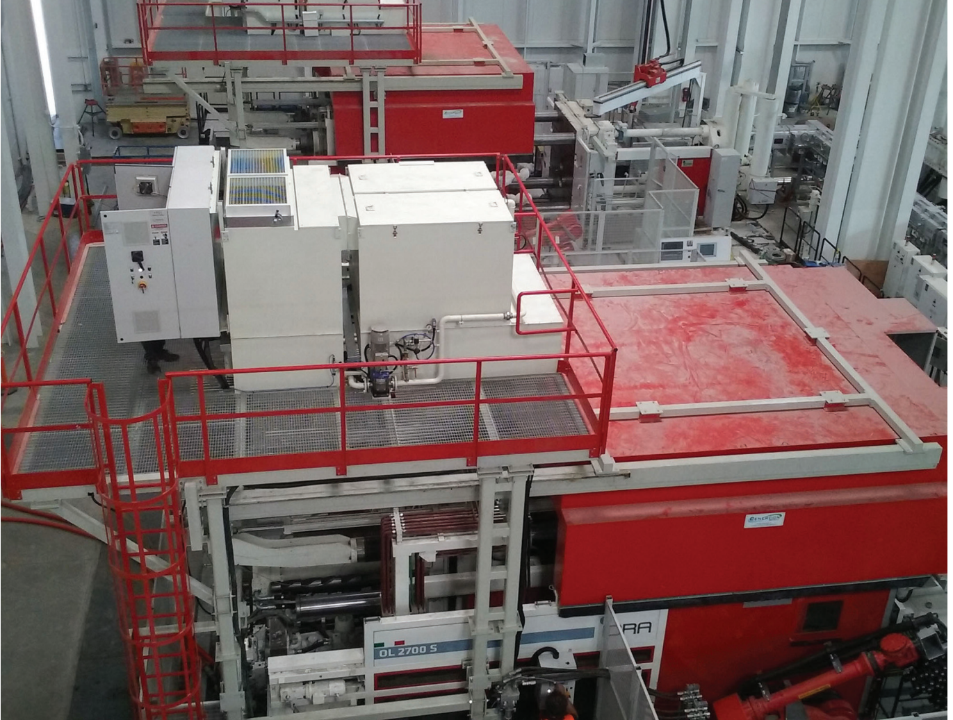
■ Hoods into two parts complete with individual ENERPRESS suction and filtration systems for recirculation of the purified air in the environment on IDRA OL4200S and OL2700S die casting machines - USA
