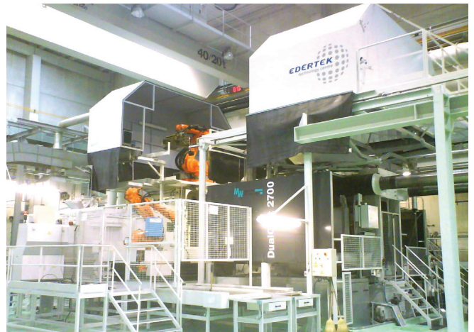
■ Hood into two parts on FRECH DUALCAST 2700 die-casting machine connected to a centralized suction and filtration system ENERPROG
